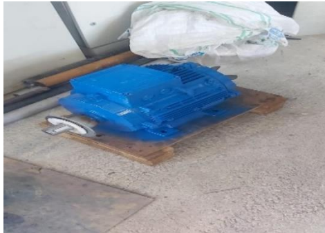
Figure 3.10 Fan Motor Ready for Assembly After Fault Rectification
