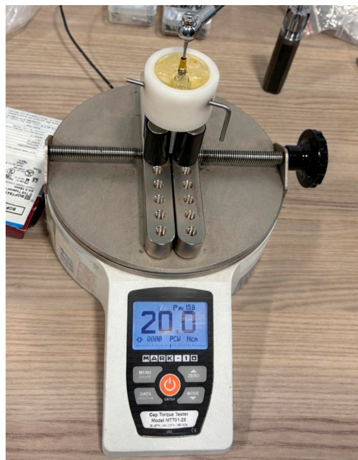
Figure 3. Digital torque meter. Every abutment screw to the manufacturer's recommended tightening torque of 20 N·cm and the reverse torque values (RTVs) were measured after they were removed from the chewing simulator.
