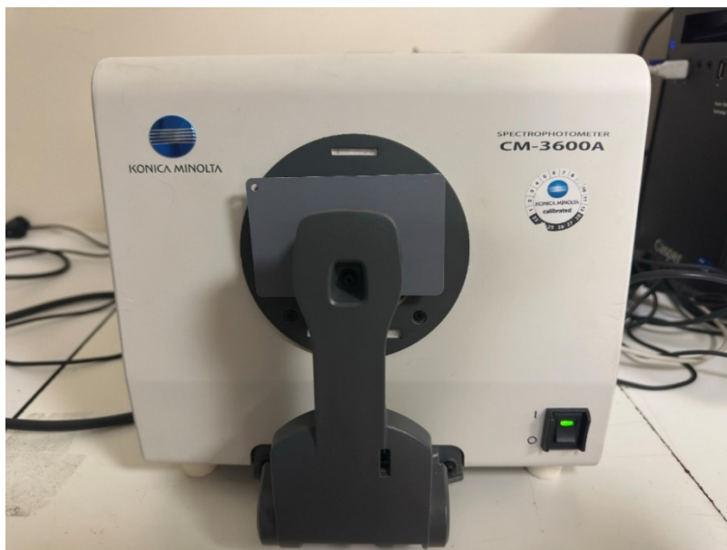
Figure 3. Spectrophotometric color measurement setup demonstrating standardized specimen positioning against an 18% gray card background.
